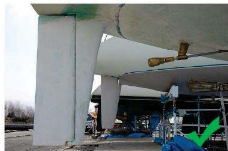
Skeg clearly visible as is propeller
