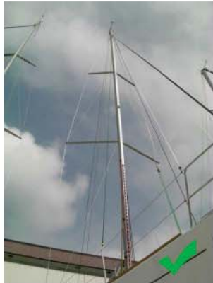
A photo of the rig showing the number of spreaders, spreader sweep and other rigging, e.g. runners/checkstays is useful
