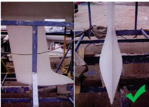
If the keel is 'low cg' (as shown above), a fore/aft view is extremely helpful
